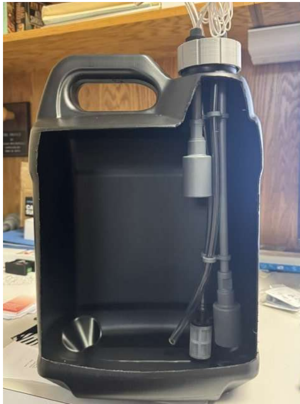
Figure 1: Side view — assembled dual-level ERECTA SWITCH configuration in cut-away 2.5-gallon detergent jug. High-level switch (5") and low-level switch (12") are physically separated, with slosh shields and tube spacers clearly visible.
