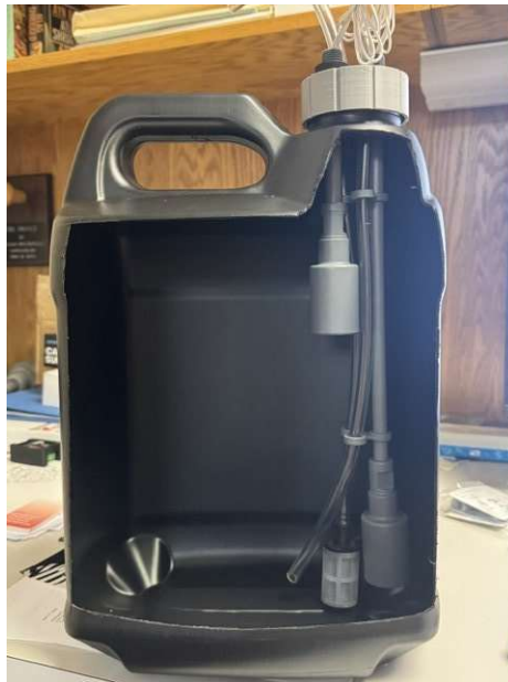
Assembled ERECTA SWITCH dual-level configuration in 2.5-gallon detergent jug
