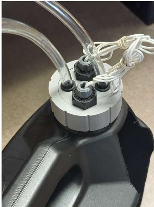
Figure 2: Top view — 4-hole custom cap with two bulkhead-mounted float switch stems and two fluid tube ports. Jam nuts and O-ring seals provide secure, leak-free, reusable mounting.
