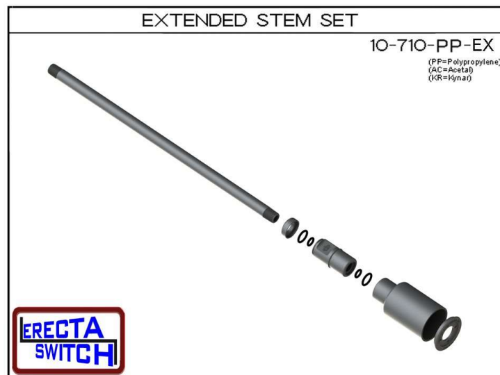
10-710-PP-EX — Exploded view of extended stem set components
