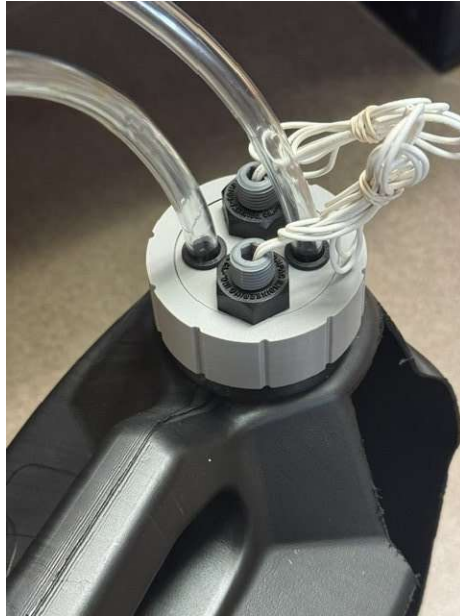
Custom 4-hole cap assembly — top view
